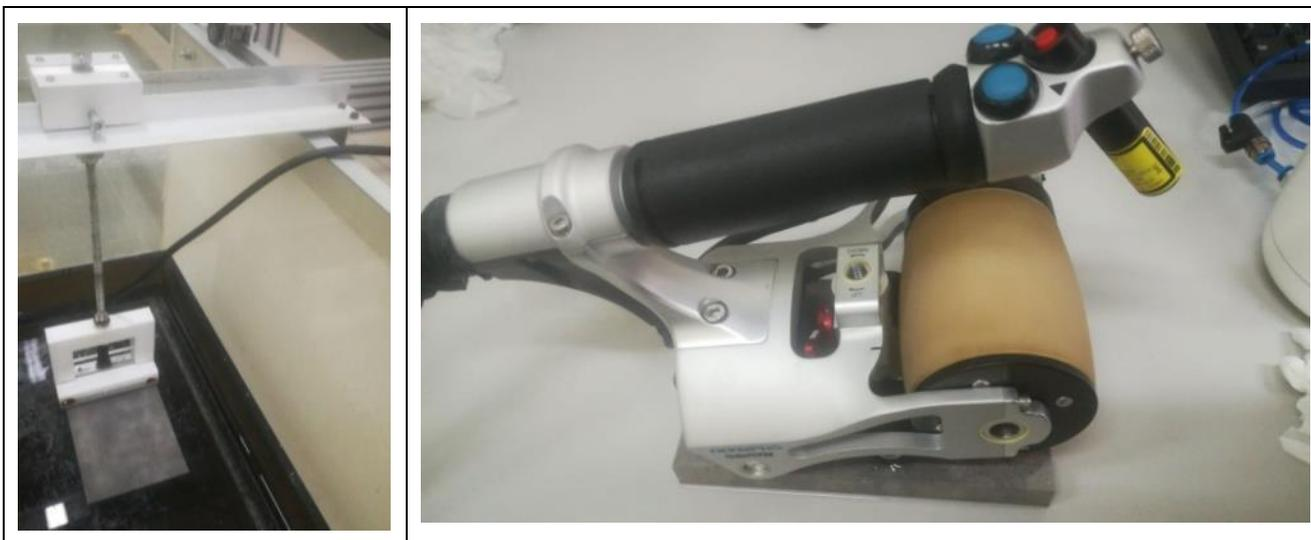
Fig. 11 setup semiautomatici con sonda phased array e Rollerform
