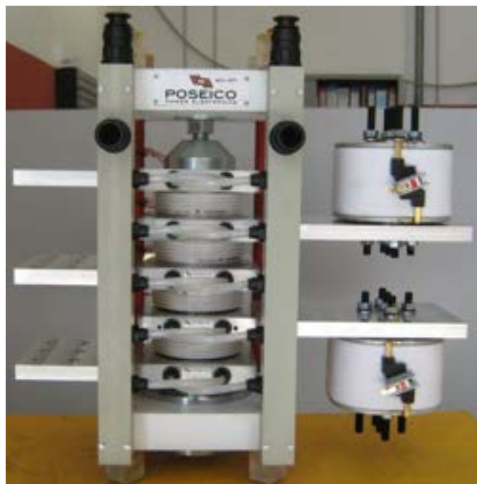
Figura 5 – Vista posteriore del CS1 power assembly.
