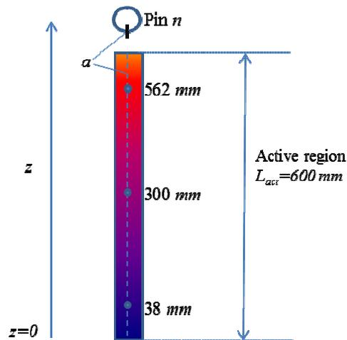
*Figure.11: Wall Embedded TCs locations for pins n. 2,4,6,7,9,16,18,19.*
