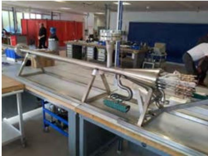
*Figure.10: Fuel pin bundle simulator assembled before installation.*
