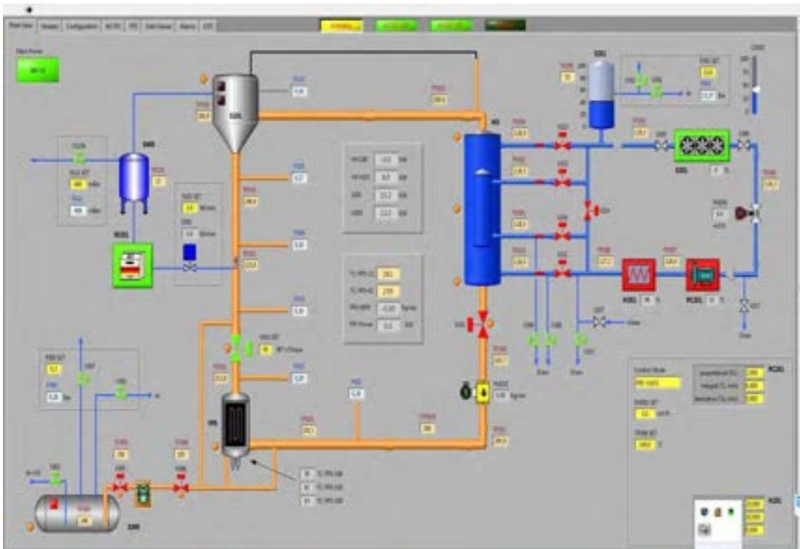
Figure.15: Remote control panel of the NACIE-UP facility
