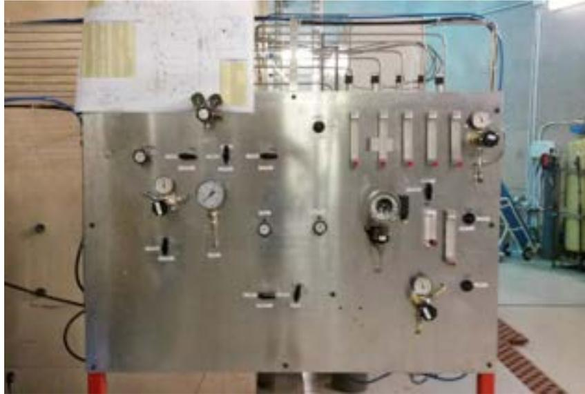
*Figure.14: Manual panel for the gas system control*
