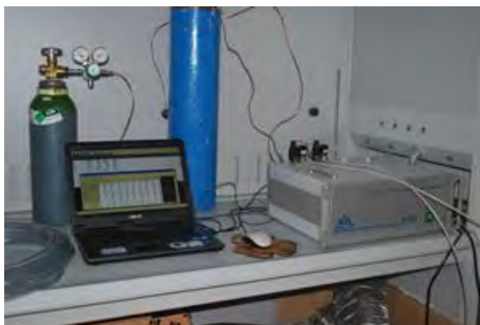
Figura 15-16. Micro gascromatografo SRA Instruments R-3000 Rack 19-inch.
