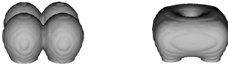
Figure 4.15: Simulation of bubble detachment from a wall in pool boiling (4)
