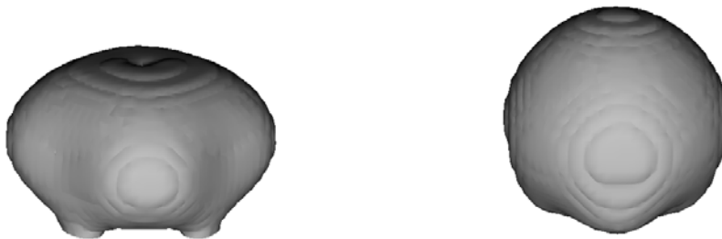
Figure 4.16: Simulation of a bubble detachment from a wall in pool boiling (5)
