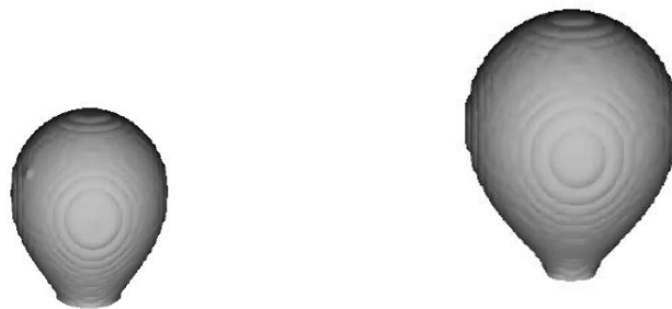
Figure 4.6: Simulation of a bubble detachment from a wall in pool boiling (5)
