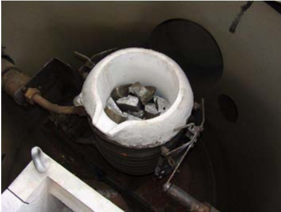
Picture 3. Raw materials are placed in the crucible of the vacuum furnace
