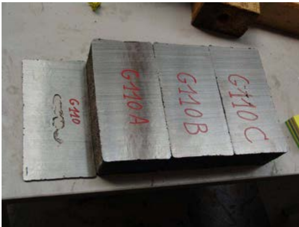
Picture 10. Illustration of the cut blocks out of an ingot
