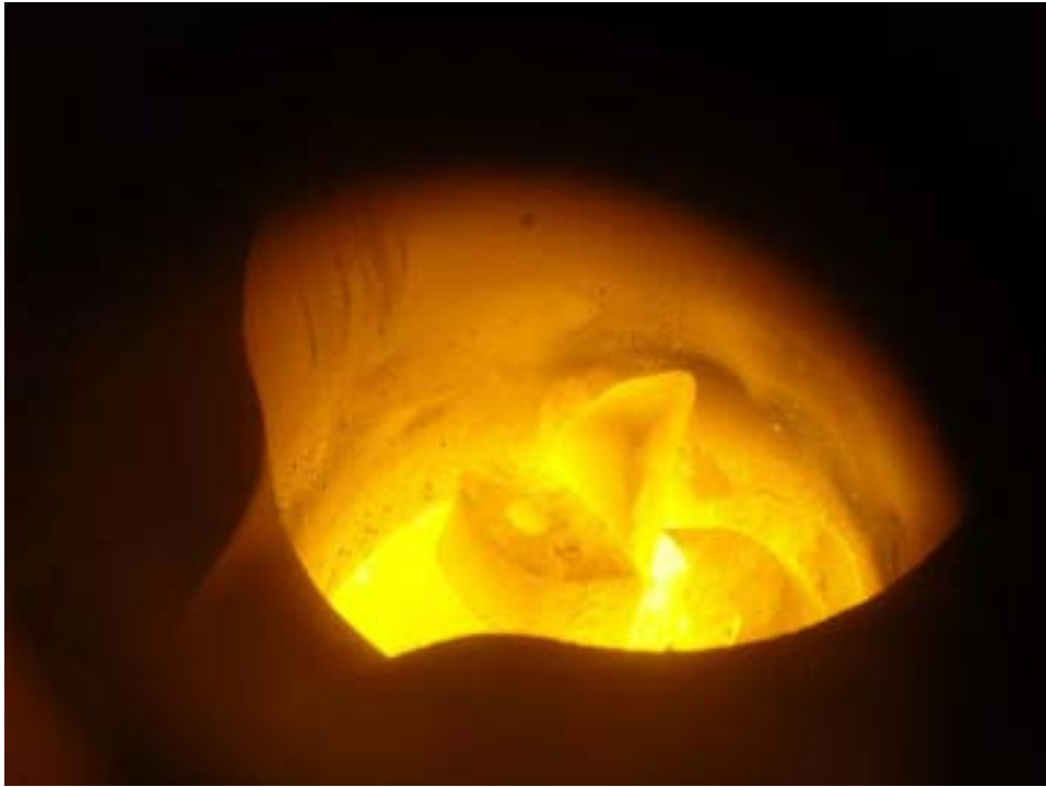
Picture 5. Raw materials heating up by induction (partially melted)
