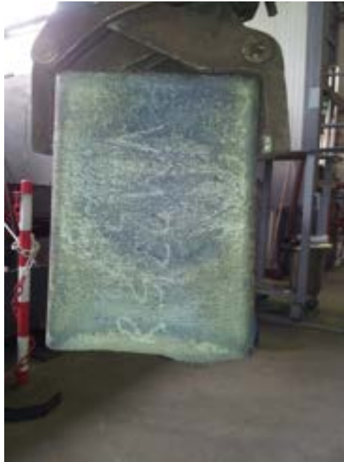
Figure 3 – VIM ingot EP302 stainless steel VM2758
