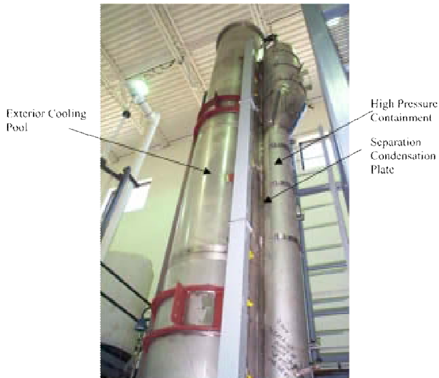
Figure 26 NuScale ITF containment
