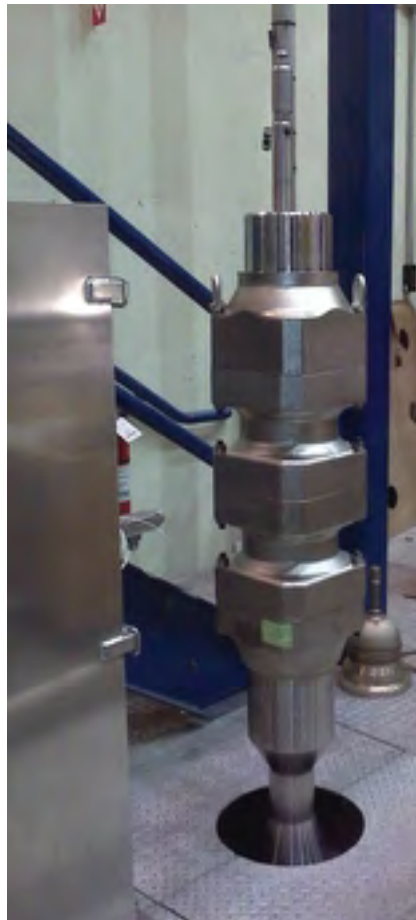
Figura 4. CRDM: Control Rod Drive Mechanism (in prova)
