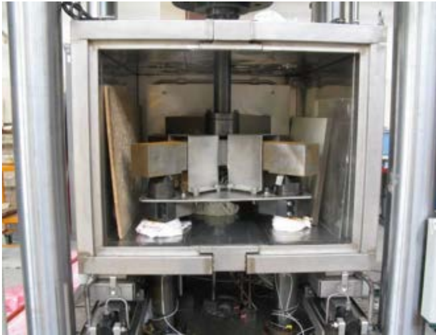
Fig. 4-6 – The 5 point bending device installed inside the thermal chamber
