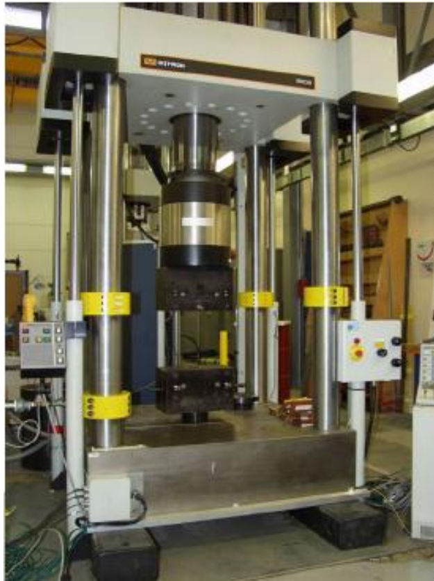
Fig. 4-4 – INSTRON 2500 kN tensile testing machine
