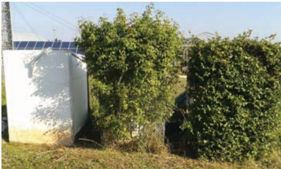
Figure 1. The three walls at the experimental field of the University of Bari. The right wall is covered with Rhynchospermum jasminoides , and the central wall with variegated Pandorea jasminoides ; the left wall is the uncovered control.
