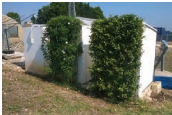
Figure 1. The experimental structures: the wall covered with R. jasminoides (right), the wall with P. jasminoides variegated (middle) and the uncovered control wall (left)
