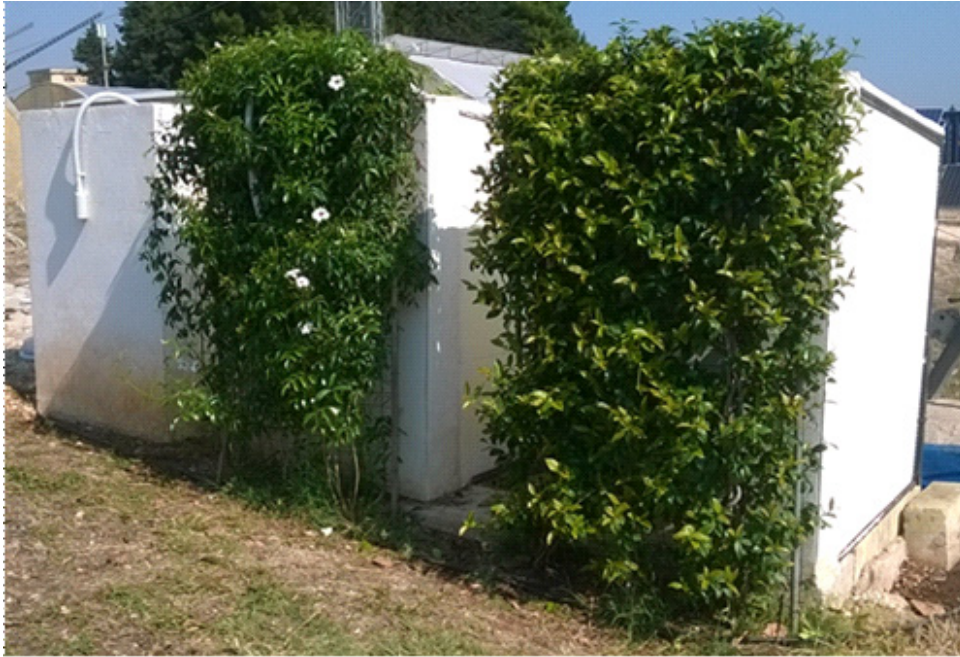
Figure 1. The three walls at the experimental field of the University of Bari; the right wall is covered with Rhynchospermum jasminoides , the central wall with Pandorea jasminoides variegated and the left wall is the uncovered control.
