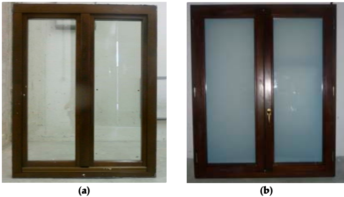
Figure 1. Wood frame window prototype Type 2 (a) with conventional double glazing units (DGUs) and (b) with aerogel in the interspace between glass layers.
