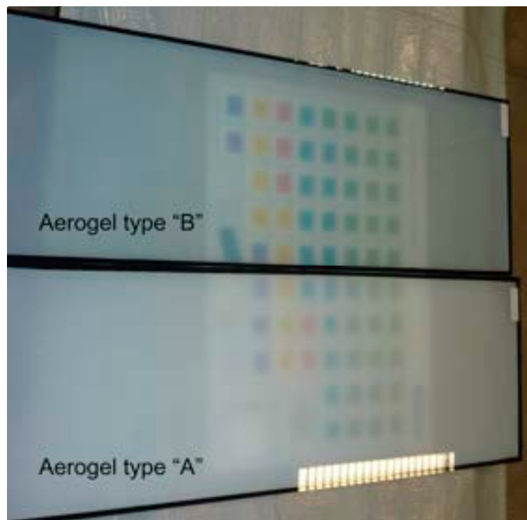
Figure 2. Glazing units with aerogel: LOW-E DGU AEROGEL with aerogel type "B" (at the top) and DGU-AEROGEL with aerogel type "A" (at the bottom).
