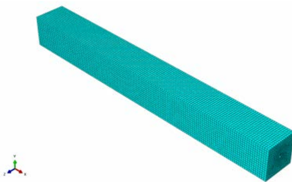
Figure 9. Portion of fluid surrounding the pin.
